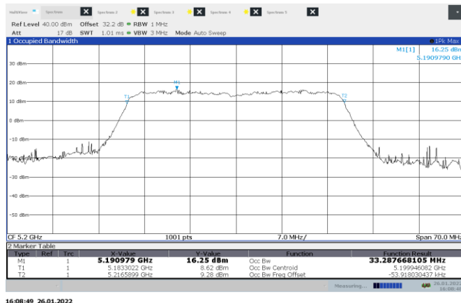
Figure 8.5-5: 99% bandwidth on 40 MHz channel, sample plot
