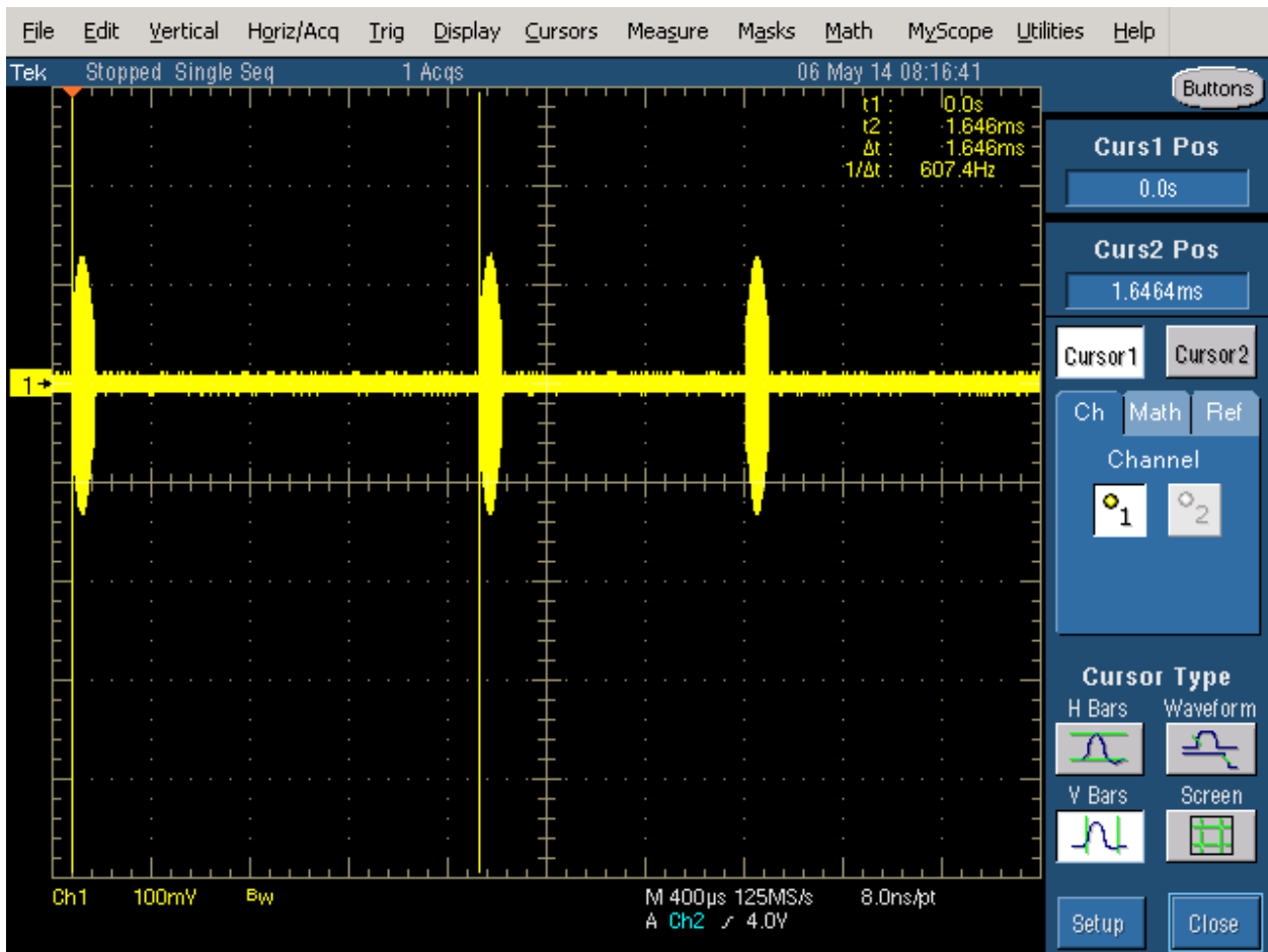
Figure 7 FCC Type 5 Radar (burst with three pulses, 1650 \mu s first period)
