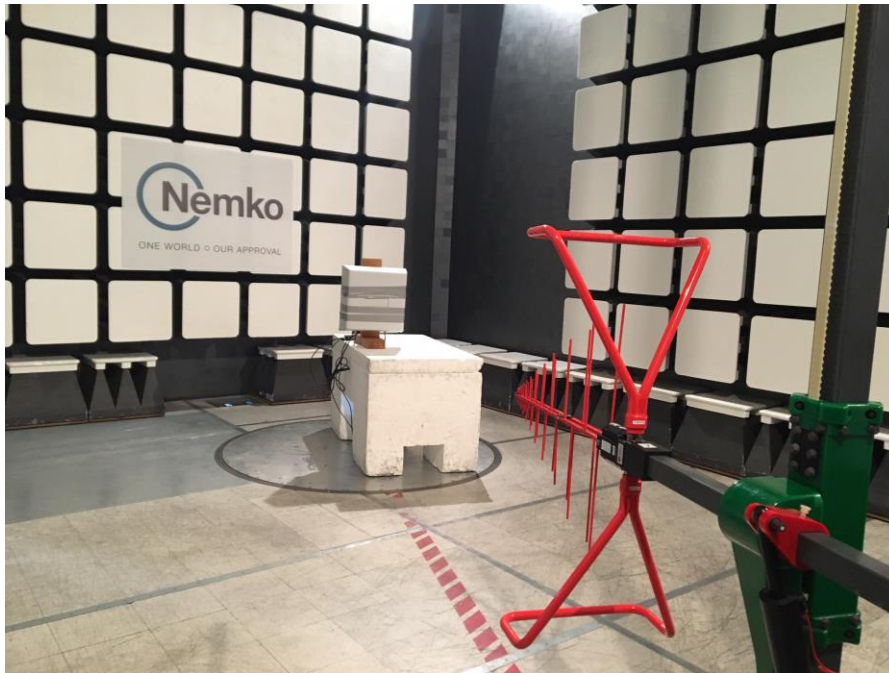
Figure 8.8-6: Radiated spurious emissions below 1 GHz with Flat antenna setup photo
