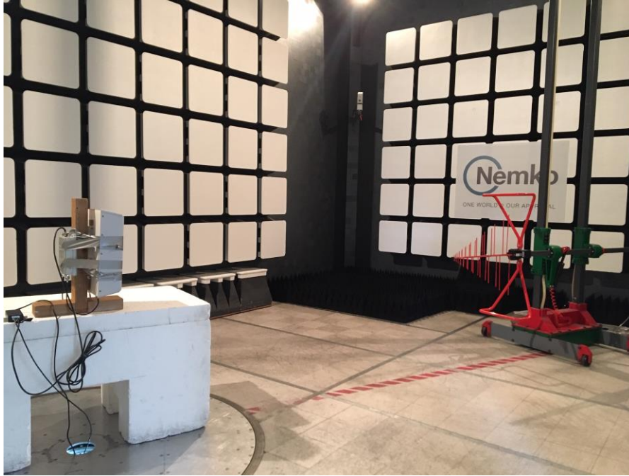
Figure 8.8-5: Radiated spurious emissions below 1 GHz with Flat antenna setup photo
