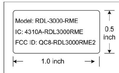
2) Location: To be placed at 'A' or 'B' on the back of the board as marked below or other redline approved location.
