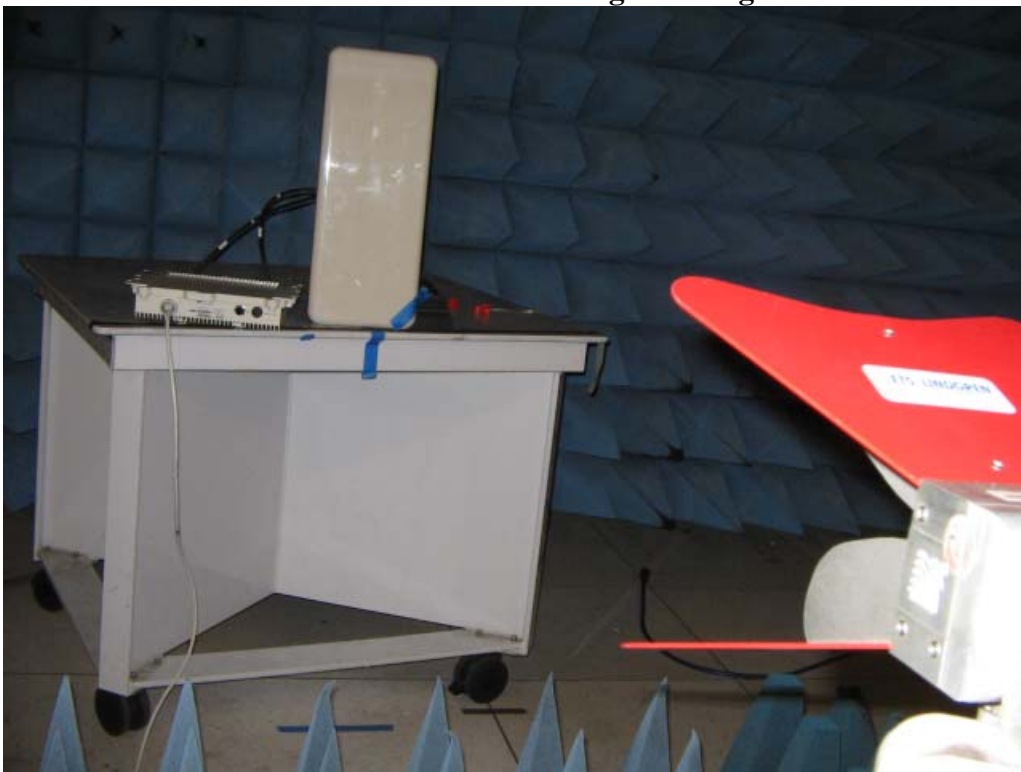
Master Device in line with radar generating antenna
