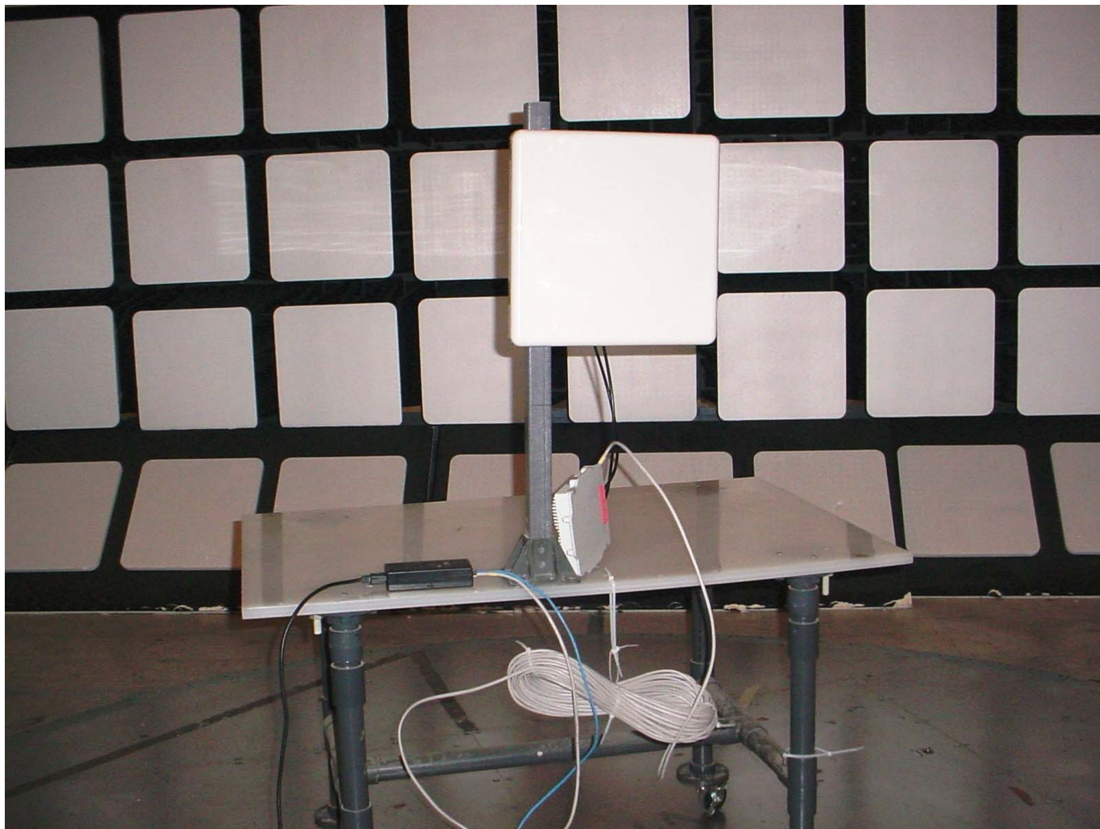
Photo #6: Test Setup for Radiated Emissions with Flat Panel Antenna, Model: A2308MFD, Gain: 23dBi
