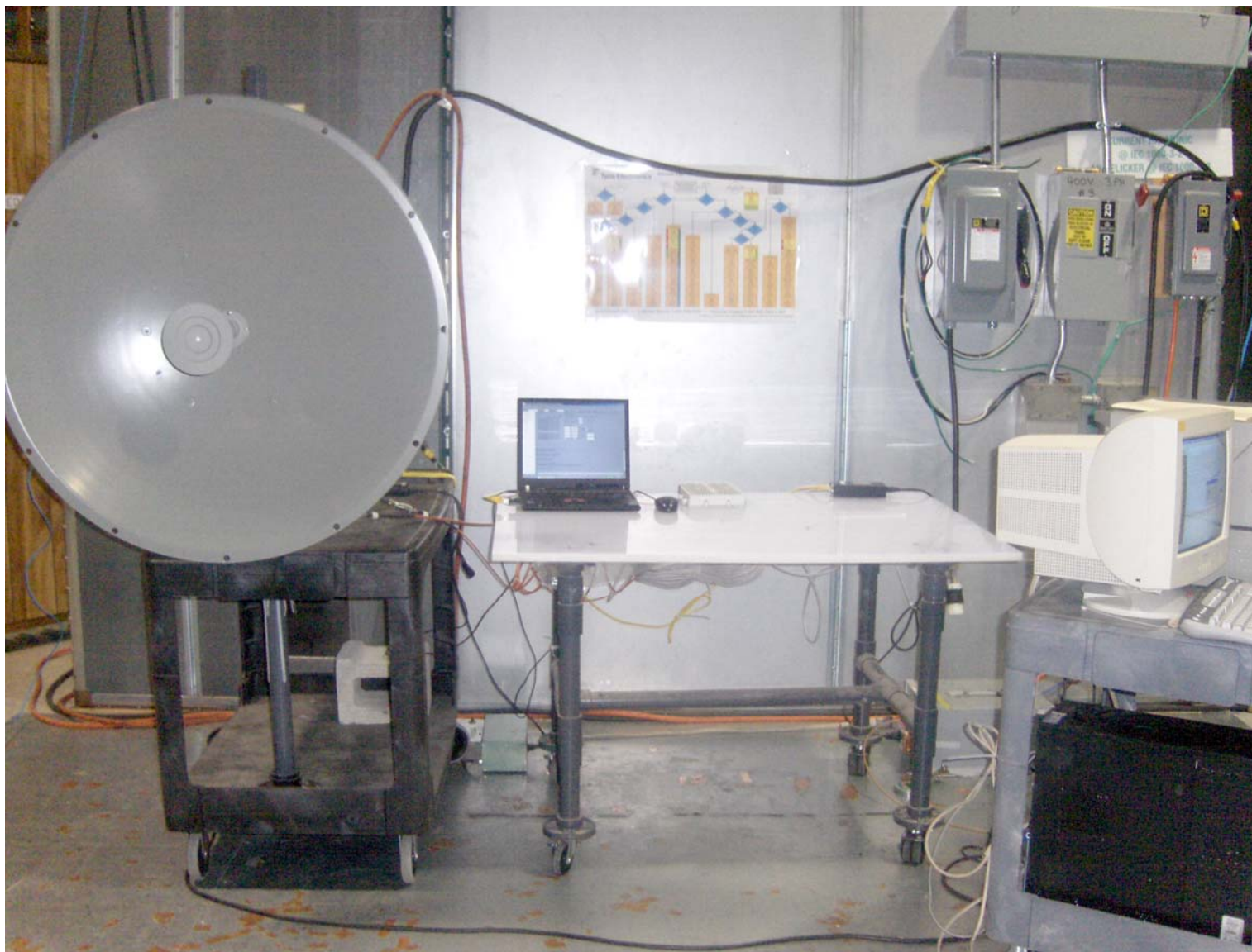
Photo #1: Test Setup for AC Powerline Conducted Emissions
