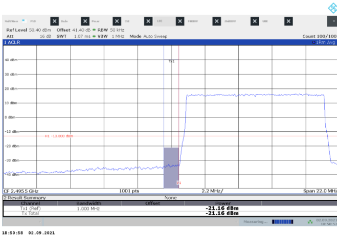
Figure 8.3-11: Band edge measurement for Ant 2 QPSK 10 MHz low channel
