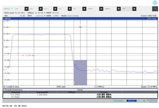
Figure 8.3-6: Band edge measurement for Ant 1 64QAM 5 MHz top channel
