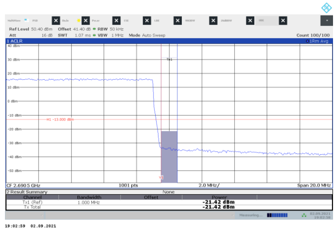
Figure 8.3-12: Band edge measurement for Ant 2 QPSK 10 MHz top channel
