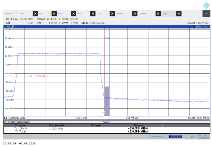
Figure 8.3-20: Band edge measurement for Ant 2 QPSK 20 MHz top channel
