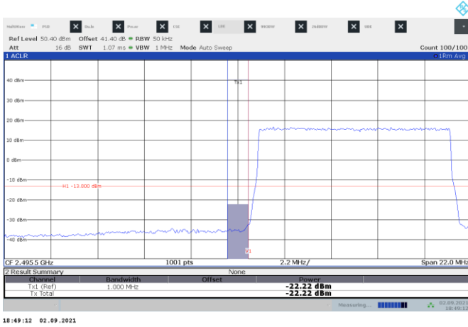
Figure 8.3-9: Band edge measurement for Ant 1 QPSK 10 MHz low channel
