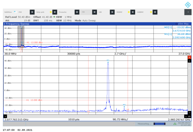
Figure 8.3-32: Conducted spurious emissions at Ant 2 64QAM 5 MHz mid channel
