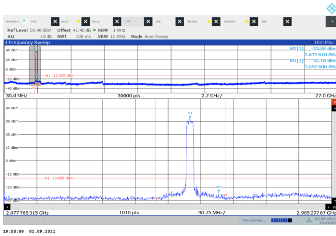
Figure 8.3-55 Conducted spurious emissions at Ant 2 QPSK 20 MHz mid channel
