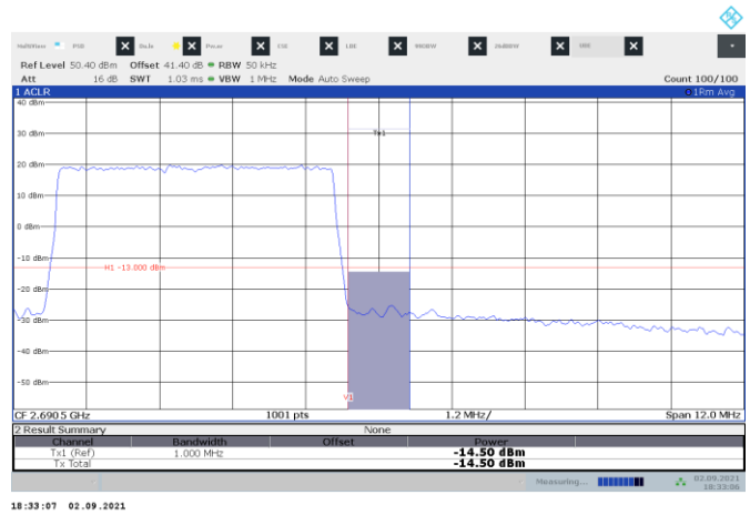
Figure 8.3-4: Band edge measurement for Ant 2 QPSK 5 MHz top channel
