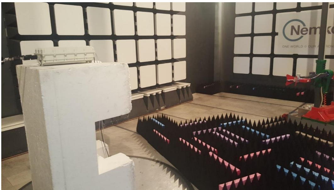
Figure 3.5-2: EUT Set-up for Radio Compliance Testing – above 1 GHz
