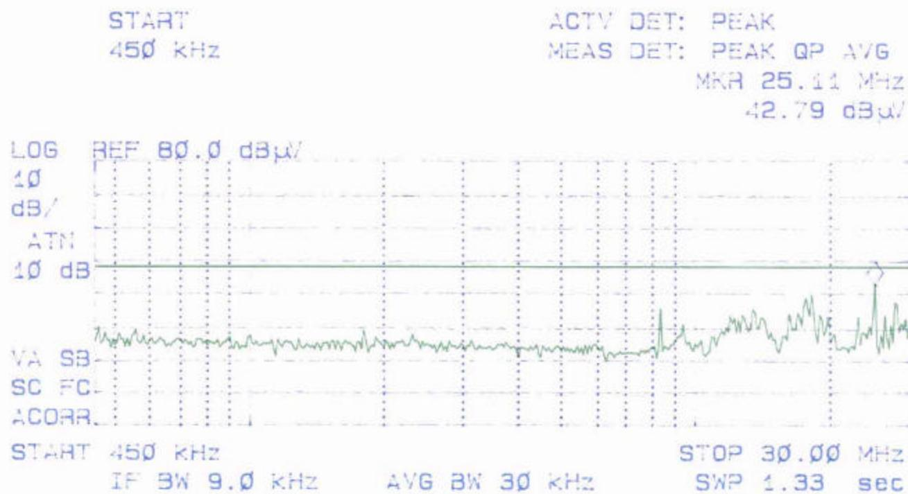
AC Powerline Conducted Emissions at "Neutral AC Line
