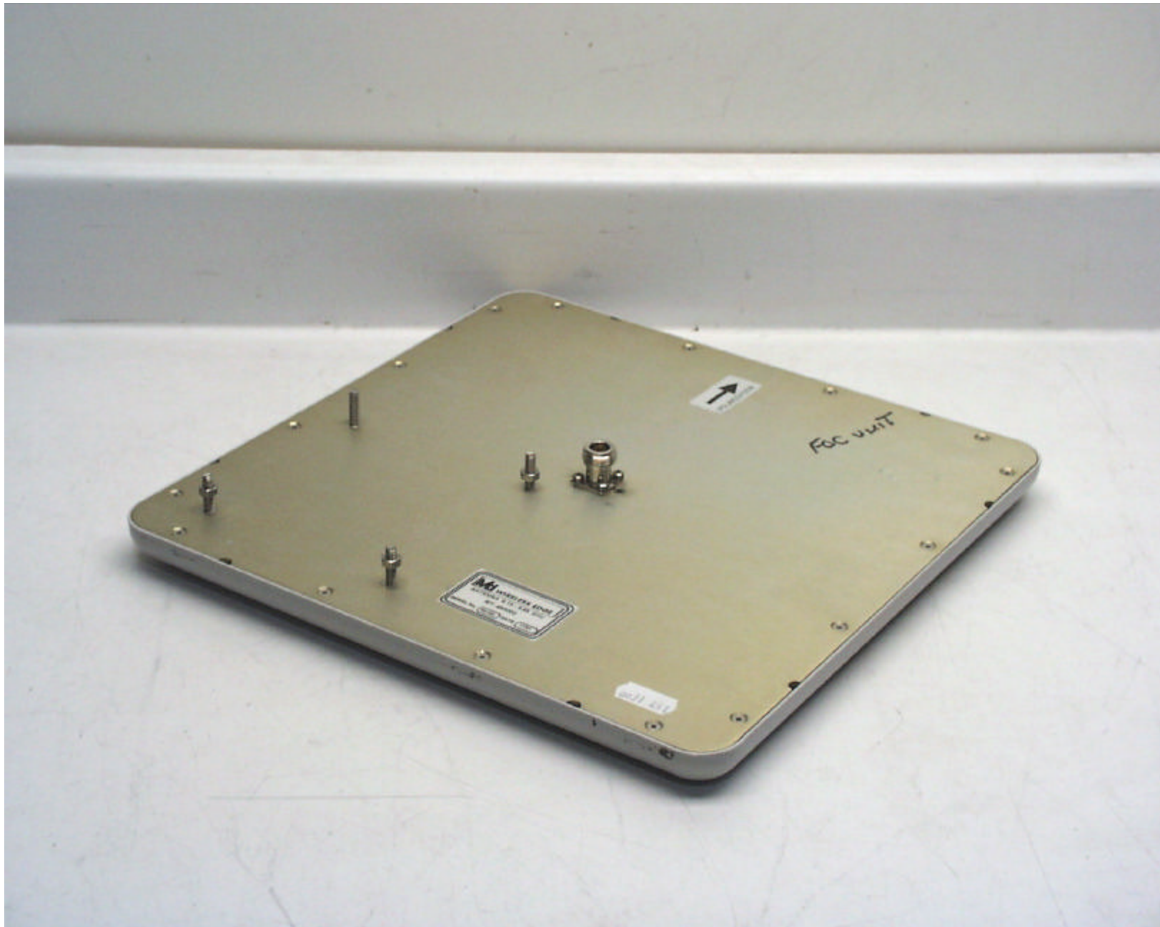
MTI Wireless Edge Antenna, P/N: 485002, Gain: 23 dBi (Back)
