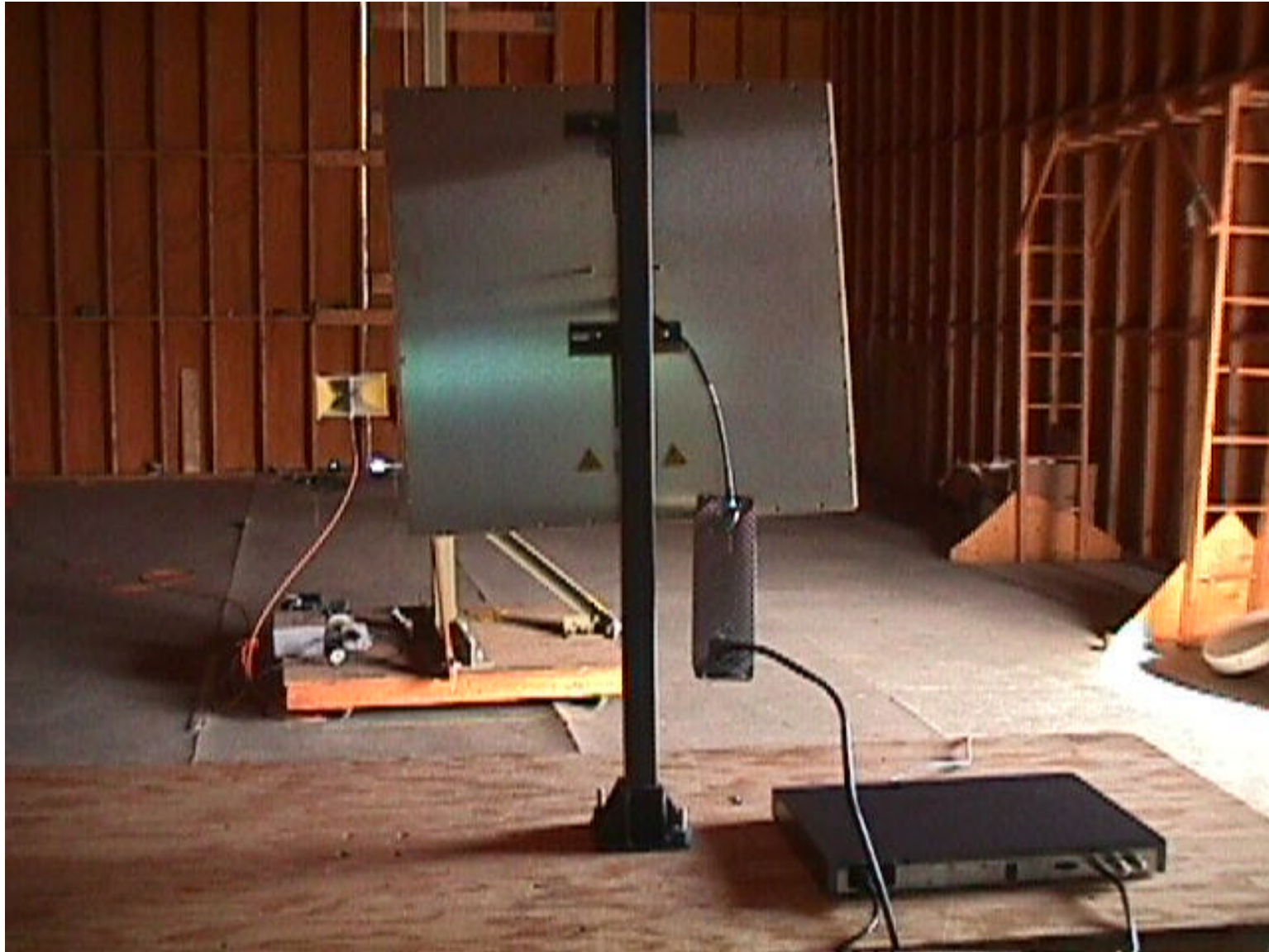
Redline AN-50 SYSTEM, MODEL AN50S with MTI Wireless Edge 28 dBi Antenna, P/N: 486001
