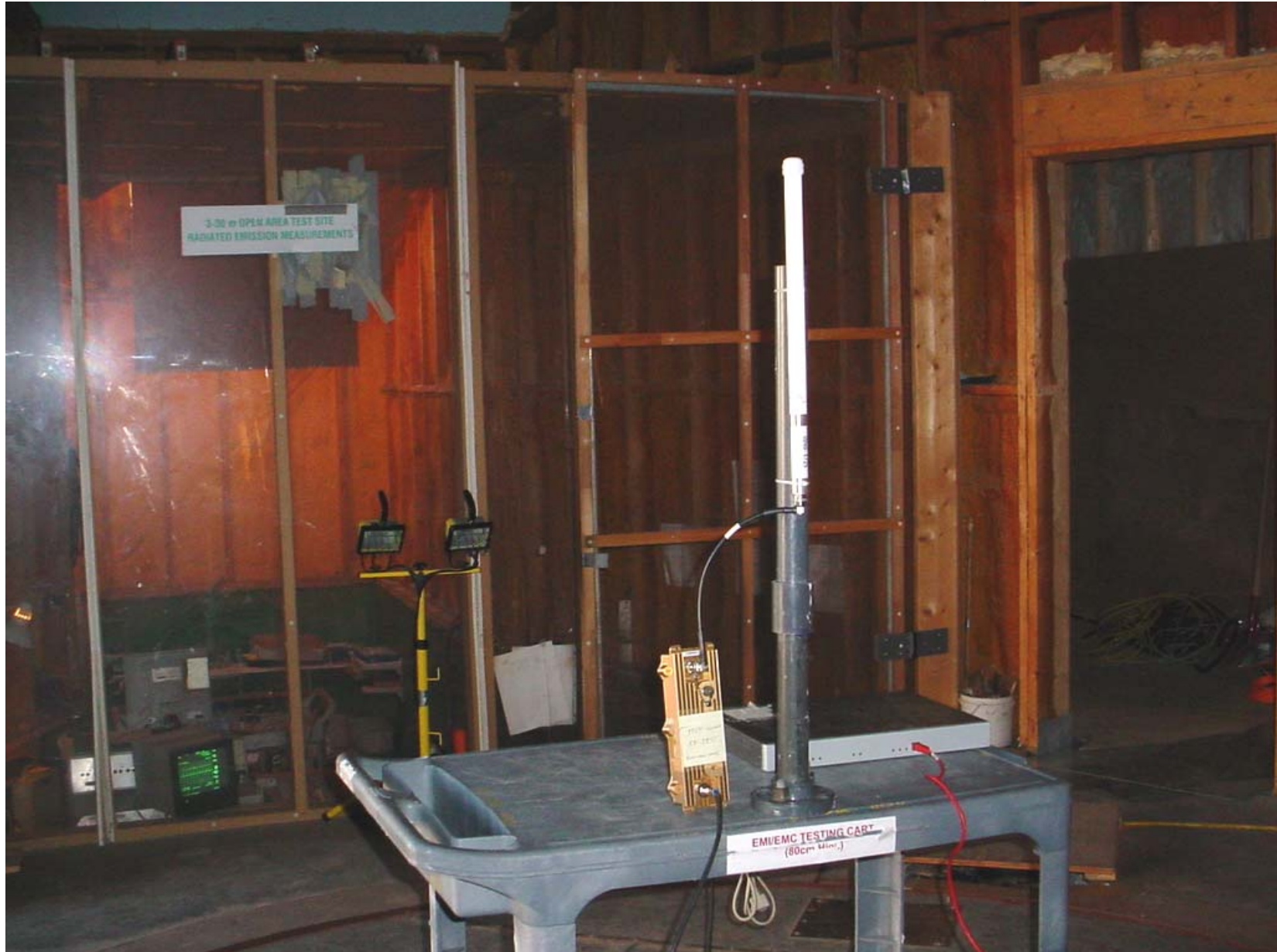
Test Setup #1: Transmitter Radiated Emissions Model AN-30E with Mobile Mark Omni Directional Antenna, Model No.: ODN9-5725, Gain: 9 dBi
