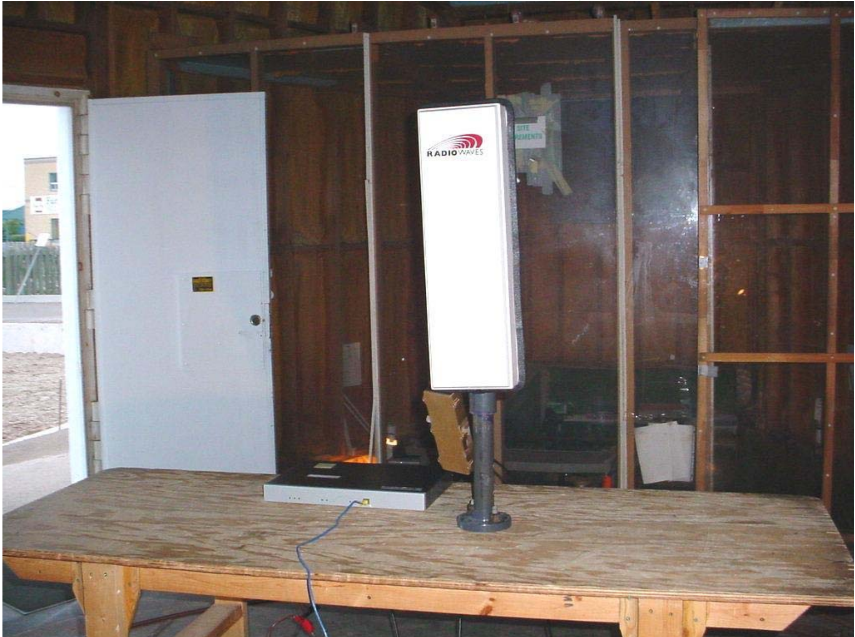
Test Setup #3: Transmitter Radiated Emissions Model AN-30E with Radiowave Antenna Model SEC-55V-60-17, Gain: 17 dBi
