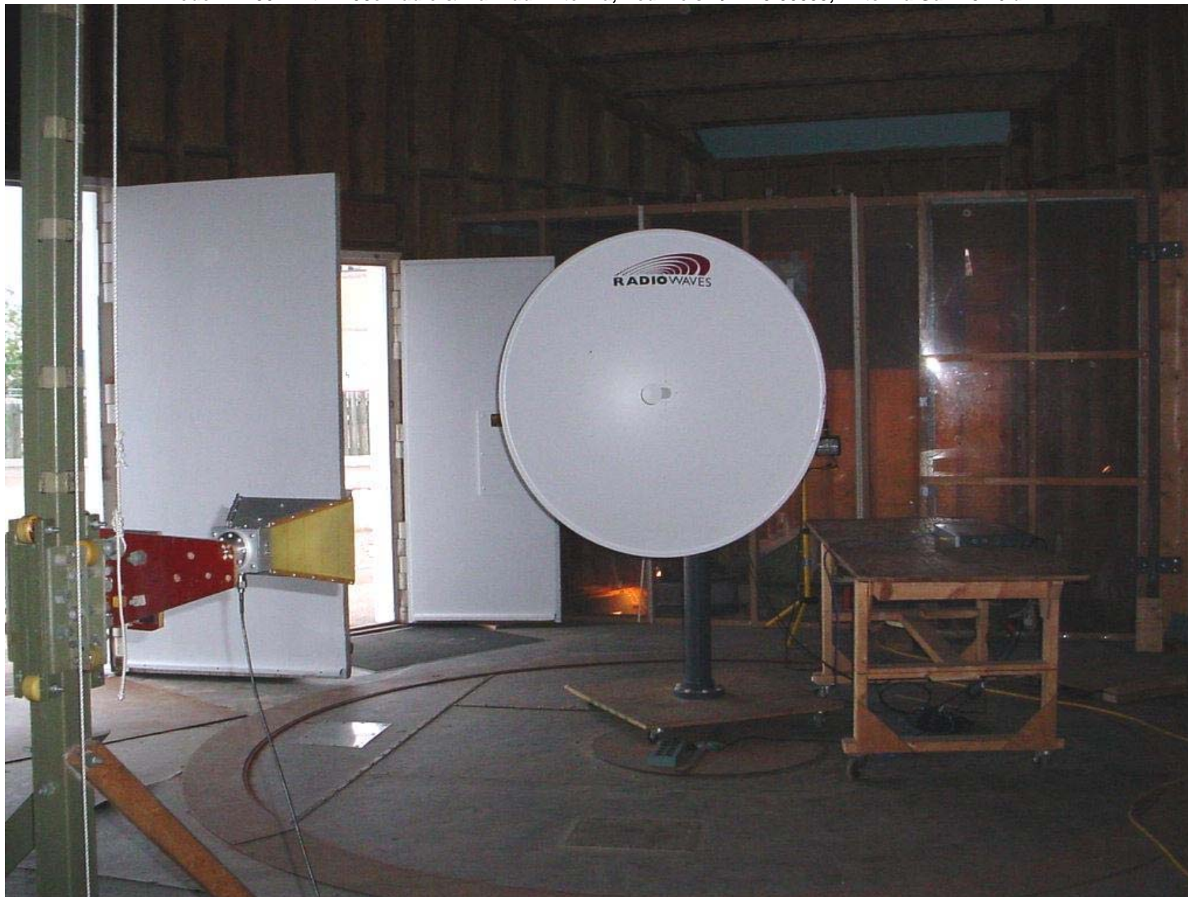
Test Setup #5: Transmitter Radiated Emissions Model AN-30E with T-58e Radio & MaxRad Antenna, Redline's P/N: 48-00033, Antenna Gain: 34.6 dBi
