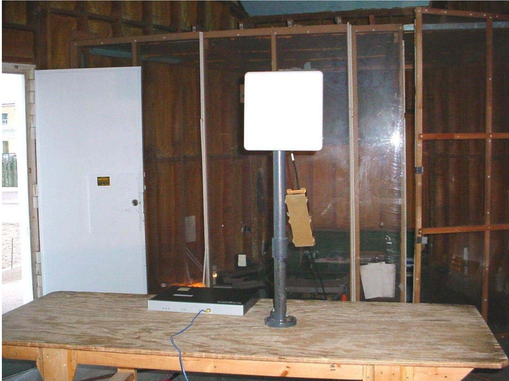
Test Setup #2: Transmitter Radiated Emissions Model AN-30E with MTI Omni Directional Antenna, Model No.: 484026, Gain: 15 dBi
