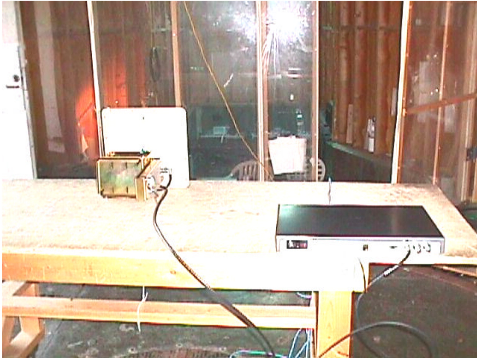
Test Setup for Model AN-50 with Model MT-585002, 23 dBi Gain Antenna
