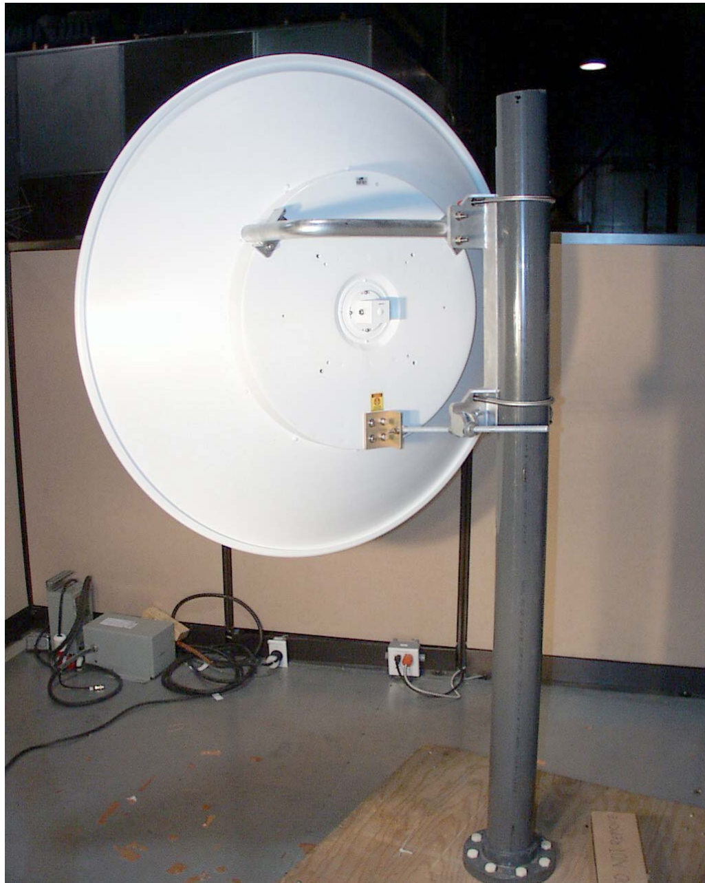
Radiowave Antenna Model SP4-5.2NS, Gain: 34.8 dBi (maximum gain within its family)
