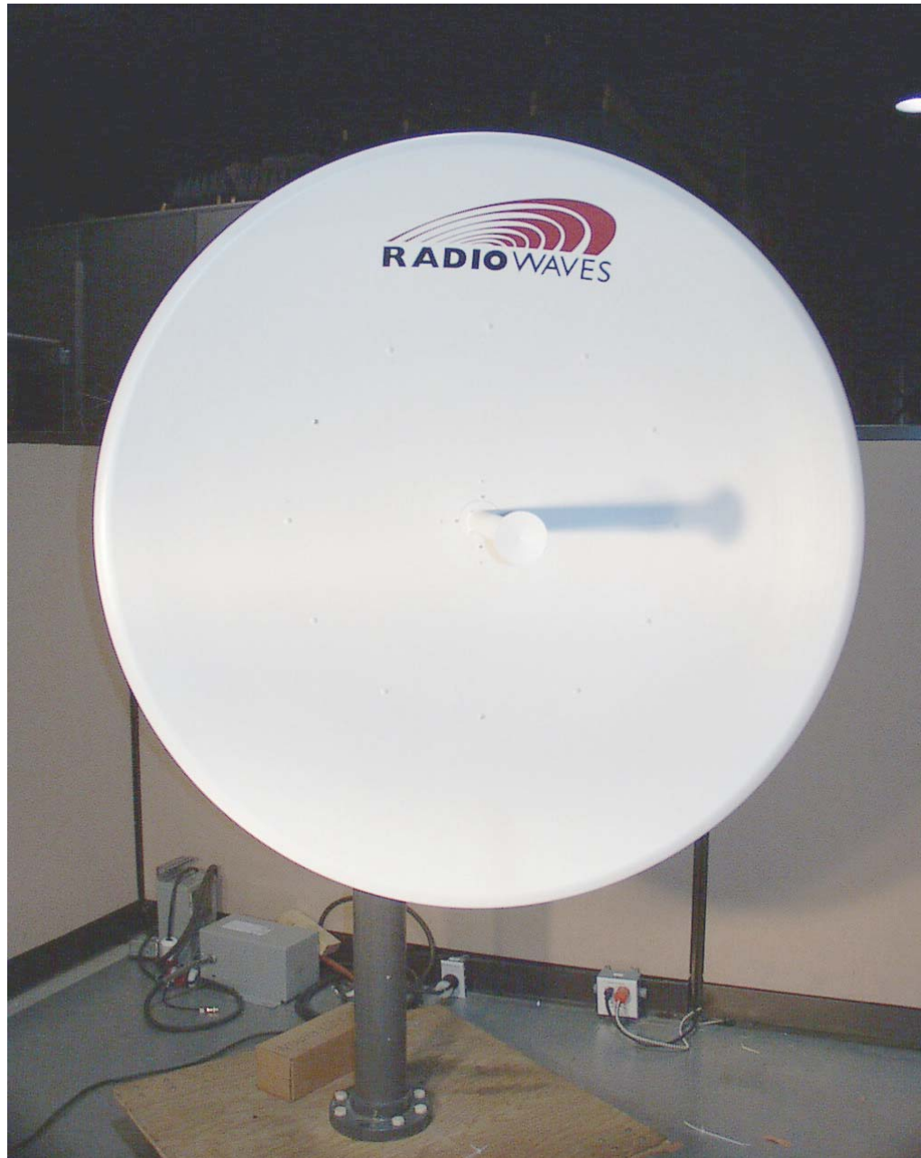
Radiowave Antenna Model SP4-5.2NS, Gain: 34.8 dBi (maximum gain within its family)
