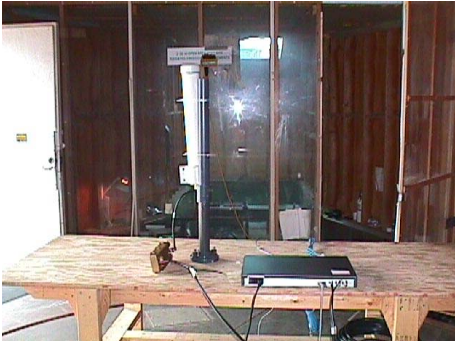
Plot # 12: Radiated Emissions Measurements at 3m Distance Tongyu Antenna Model TDJ-5818AM-60, Gain: 18.0 dBi (maximum gain within its family)
