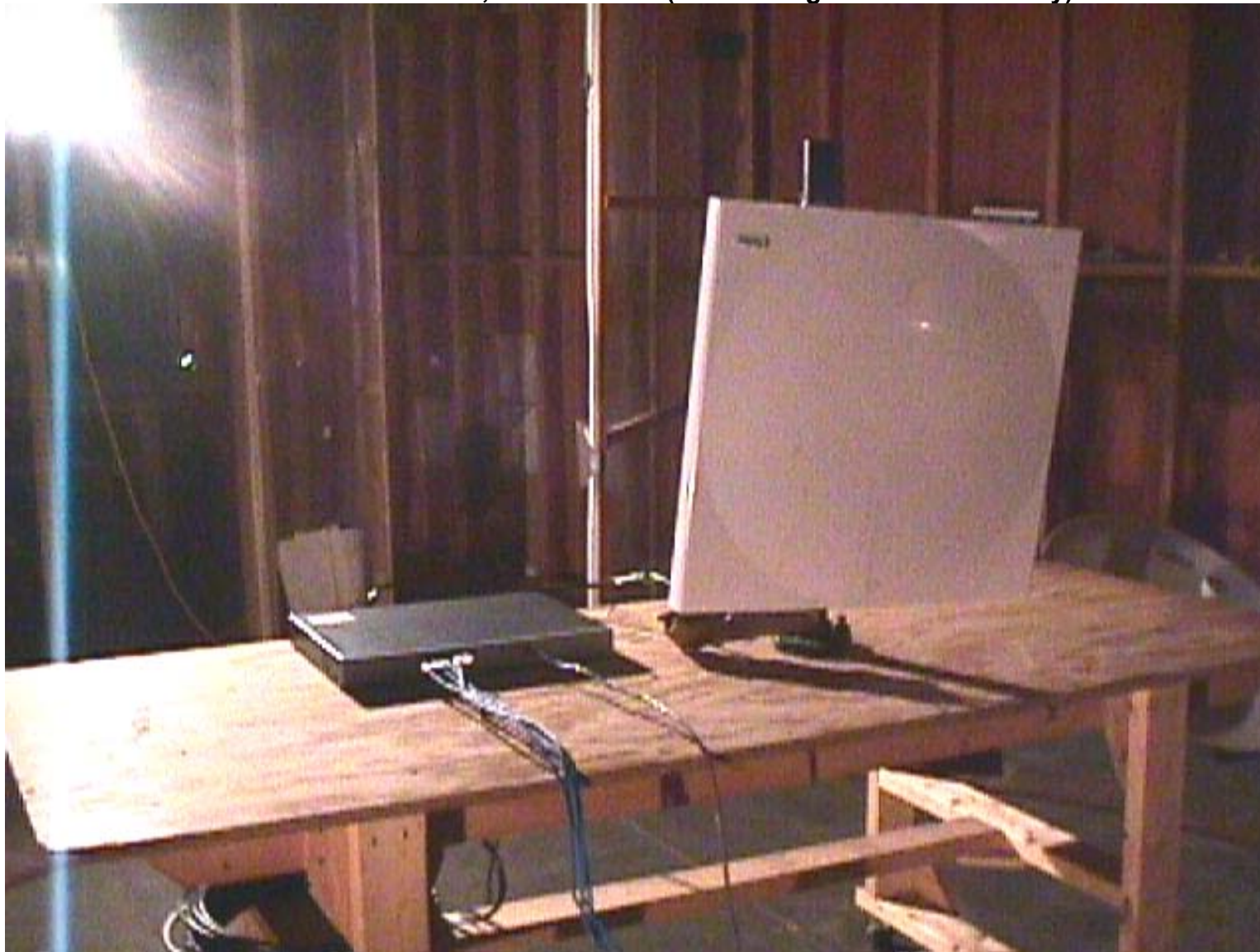
Plot # 3: Radiated Emissions Measurements at 3m Distance with MTI Antenna Model 486001, Gain: 28 dBi (maximum gain within its family)
