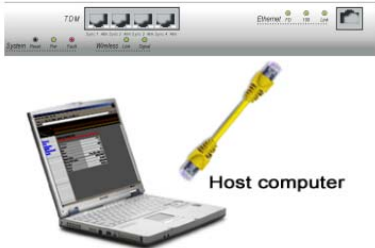
Figure 11: AN-30 Terminal Connected To Host Computer
