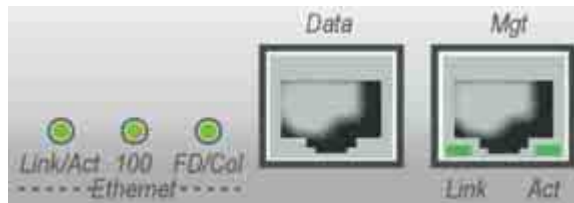
Figure 11: System - AN-100U/UX Front Panel Ethernet LEDs and Ports
