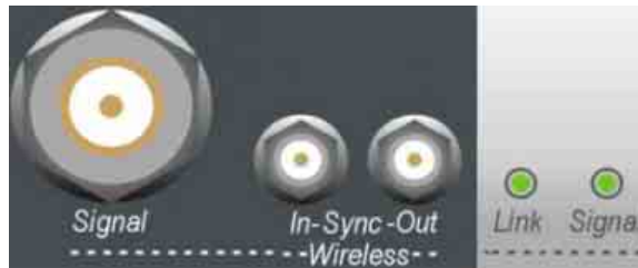
Figure 10: System - AN-100U/UX Front Panel Wireless Section
