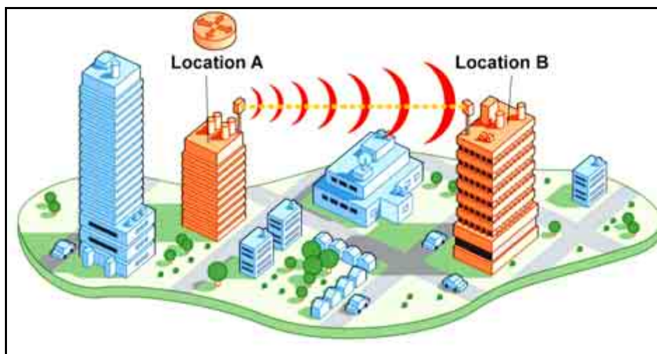
Figure 4: System - PTP Line of Sight Deployment
