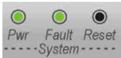
Figure 12: System - AN-100U/UX System LEDs and Reset Switch
