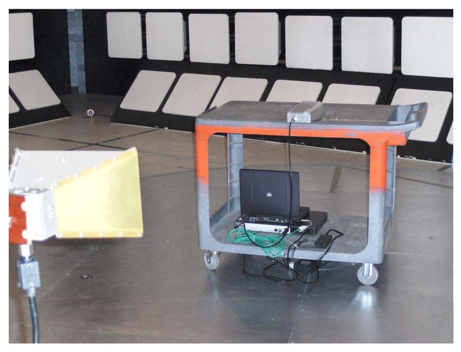
Annex 1 – Test Setup Photographs of Model AN-100U with TB3638F7 Radio FCC ID: QC8-AN100UA
