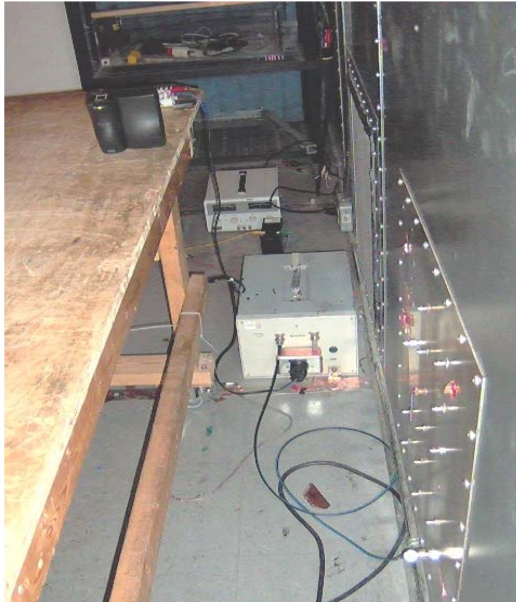
Photo #2: Powerline Conducted Emission Measurements
