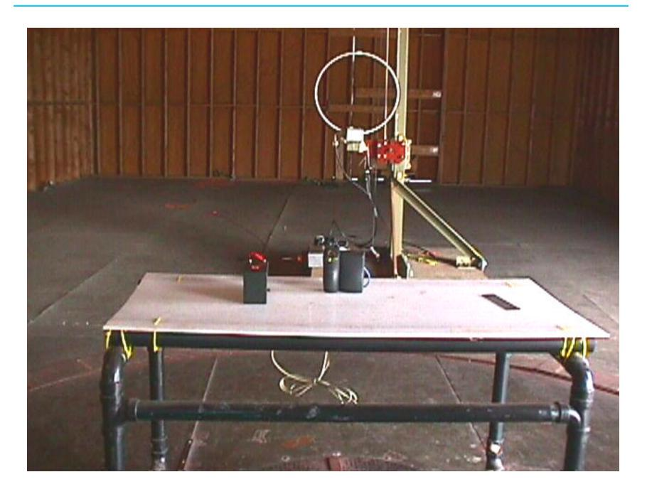
EMISSIONS MEASUREMENTS (EUT WAS PLACED IN 3 DIFFERENT ORTHOGONAL DIRECTIONS) V-SMART, Model V-SMART, A, H
