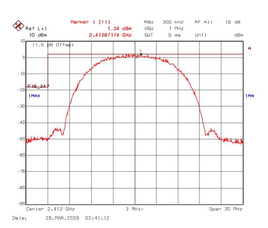
Plot 5.7.5.1.1 Band-Edge RF Conducted Emissions, 802.11b Mode Low End of Frequency Band 2412 -2462 MHz
