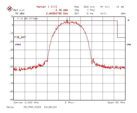
Plot 5.7.5.1.3 Band-Edge RF Conducted Emissions, 802.11g Mode Low End of Frequency Band 2412 -2462 MHz
