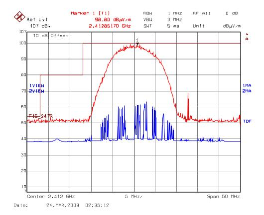
Plot 5.8.5.1.3 Band-Edge RF Radiated Emissions @ 3 m High End of Frequency Band; Test Frequency: 2462 MHz Rx Antenna Orientation: Horizontal
