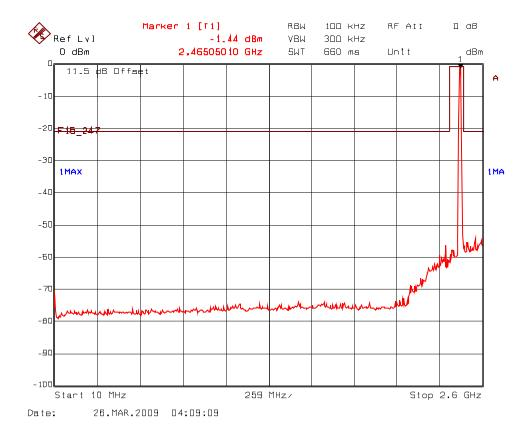
Plot 5.7.5.2.3(ii) Spurious RF Conducted Emissions, 802.11b Mode Transmitter Frequency: 2462 MHz
