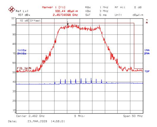
Plot 5.8.5.1.8 Band-Edge RF Radiated Emissions @ 3 m High End of Frequency Band; Test Frequency: 2462 MHz Rx Antenna Orientation: Vertical
