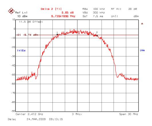
Plot 5.5.5.5 6 dB Bandwidth Frequency: 2437 MHz; Modulation: DQPSK at 2 Mbps
