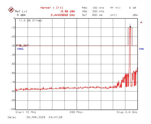
Plot 5.7.5.2.5(ii) Spurious RF Conducted Emissions, 802.11g Mode Transmitter Frequency: 2437 MHz
