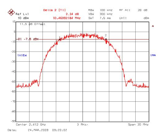
Plot 5.5.5.8 6 dB Bandwidth Frequency: 2437 MHz; Modulation: CCK at 11 Mbps
