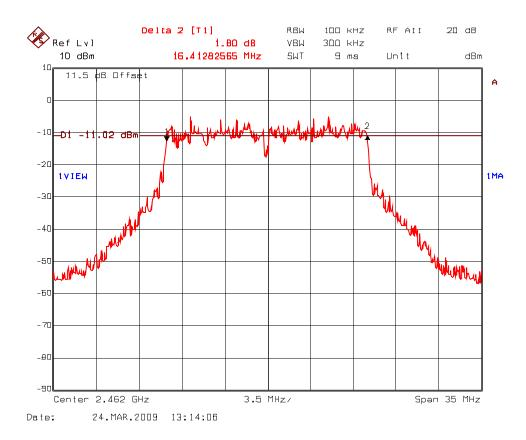
Plot 5.5.5.19 6 dB Bandwidth Frequency: 2412 MHz; Modulation: 64QAM at 54 Mbps
