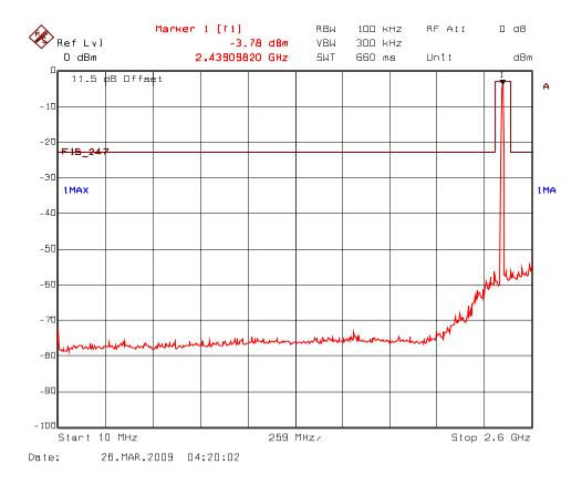
Plot 5.7.5.2.2(ii) Spurious RF Conducted Emissions, 802.11b Mode Transmitter Frequency: 2437 MHz
