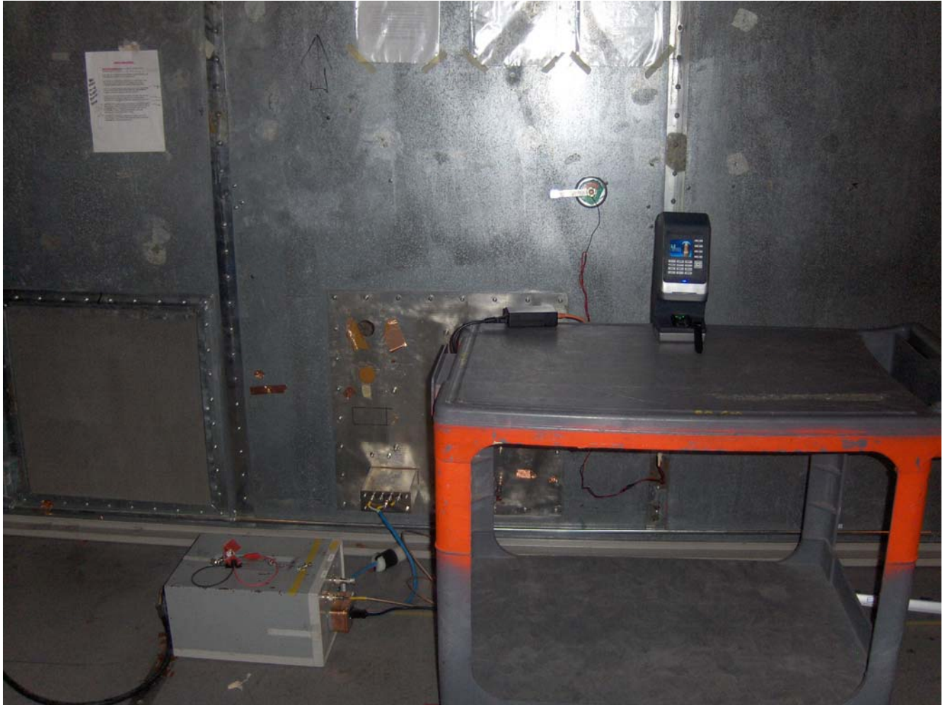
Power Line Conducted Emissions Test Configuration 2: Power over Ethernet (PoE) Injector
