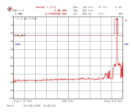
**Plot 5.7.5.2.6(ii)** Spurious RF Conducted Emissions, 802.11g Mode Transmitter Frequency: 2462 MHz
