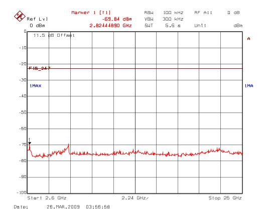
Plot 5.7.5.2.4(i) Spurious RF Conducted Emissions, 802.11g Mode Transmitter Frequency: 2412 MHz
