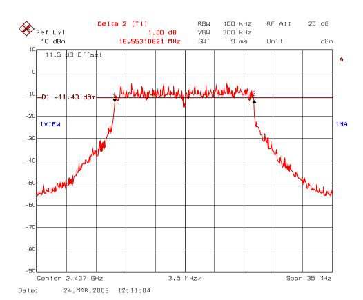
Plot 5.5.5.12 6 dB Bandwidth Frequency: 2462 MHz; Modulation: BPSK at 9 Mbps
