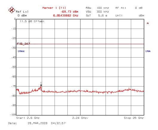
Plot 5.7.5.2.5(i) Spurious RF Conducted Emissions, 802.11g Mode Transmitter Frequency: 2437 MHz
