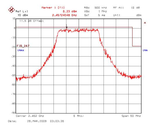
Plot 5.7.5.2.1(i) Spurious RF Conducted Emissions, 802.11b Mode Transmitter Frequency: 2412 MHz
