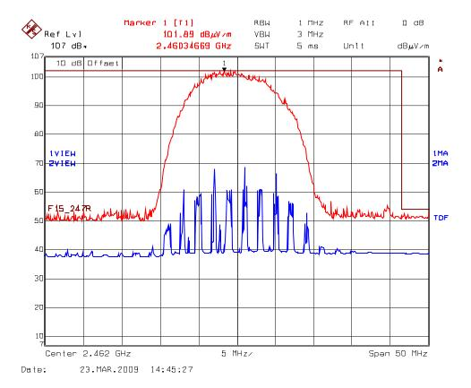
Plot 5.8.5.1.4 Band-Edge RF Radiated Emissions @ 3 m High End of Frequency Band; Test Frequency: 2462 MHz Rx Antenna Orientation: Vertical
