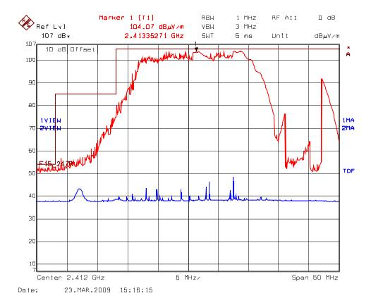
Plot 5.8.5.1.6 Band-Edge RF Radiated Emissions @ 3 m Low End of Frequency Band; Test Frequency: 2412 MHz Rx Antenna Orientation: Vertical
