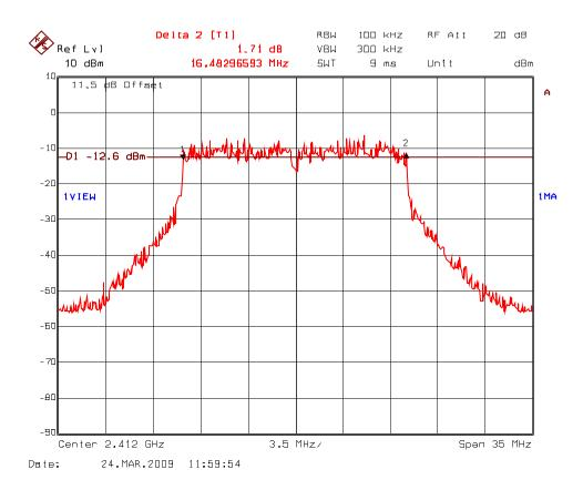
Frequency: 2437 MHz; Modulation: BPSK at 9 Mbps
