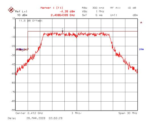
Plot 5.7.5.1.4 Band-Edge RF Conducted Emissions, 802.11g Mode High End of Frequency Band 2412 -2462 MHz
