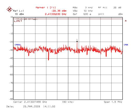
**Plot 5.9.5.5** Power Spectral Density Frequency: 2437 MHz
