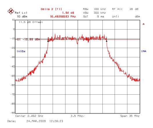
**Plot 5.5.5.13** 6 dB Bandwidth Frequency: 2412 MHz; Modulation: QPSK at 18 Mbps
