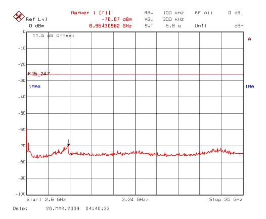
Plot 5.7.5.2.6(i) Spurious RF Conducted Emissions, 802.11g Mode Transmitter Frequency: 2462 MHz
