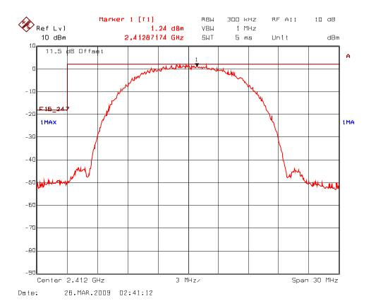
Plot 5.7.5.1.2 Band-Edge RF Conducted Emissions, 802.11b Mode High End of Frequency Band 2412 -2462 MHz
