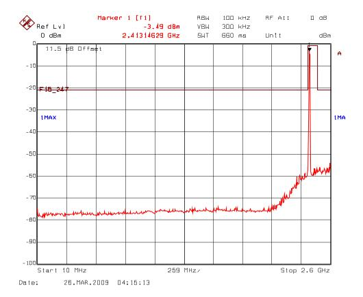
Plot 5.7.5.2.1(ii) Spurious RF Conducted Emissions, 802.11b Mode Transmitter Frequency: 2412 MHz
