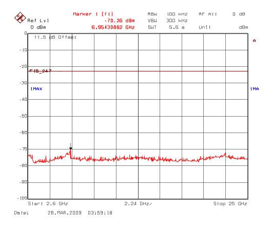
Plot 5.7.5.2.3(i) Spurious RF Conducted Emissions, 802.11b Mode Transmitter Frequency: 2462 MHz
