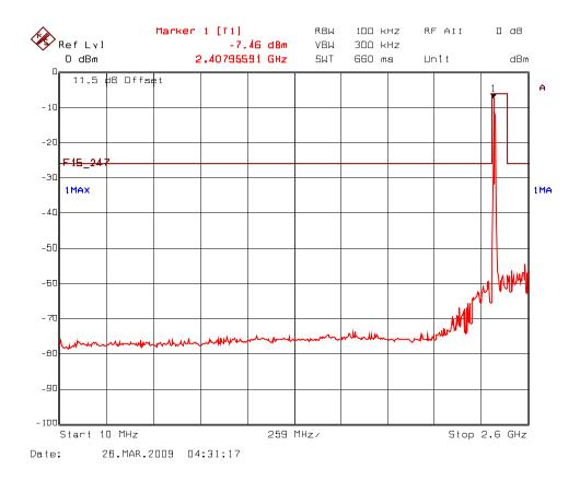
Plot 5.7.5.2.4(ii) Spurious RF Conducted Emissions, 802.11g Mode Transmitter Frequency: 2412 MHz
