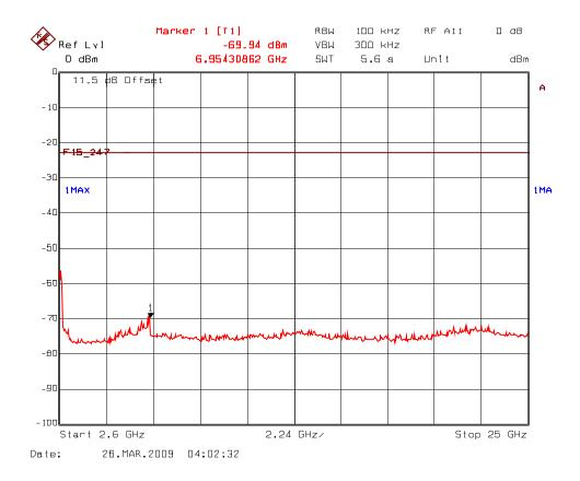
Plot 5.7.5.2.2(i) Spurious RF Conducted Emissions, 802.11b Mode Transmitter Frequency: 2437 MHz
