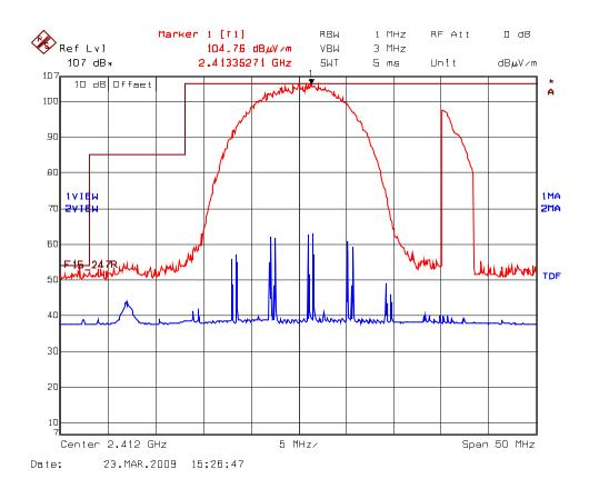
Plot 5.8.5.1.2 Band-Edge RF Radiated Emissions @ 3 m Low End of Frequency Band; Test Frequency: 2412 MHz Rx Antenna Orientation: Vertical
