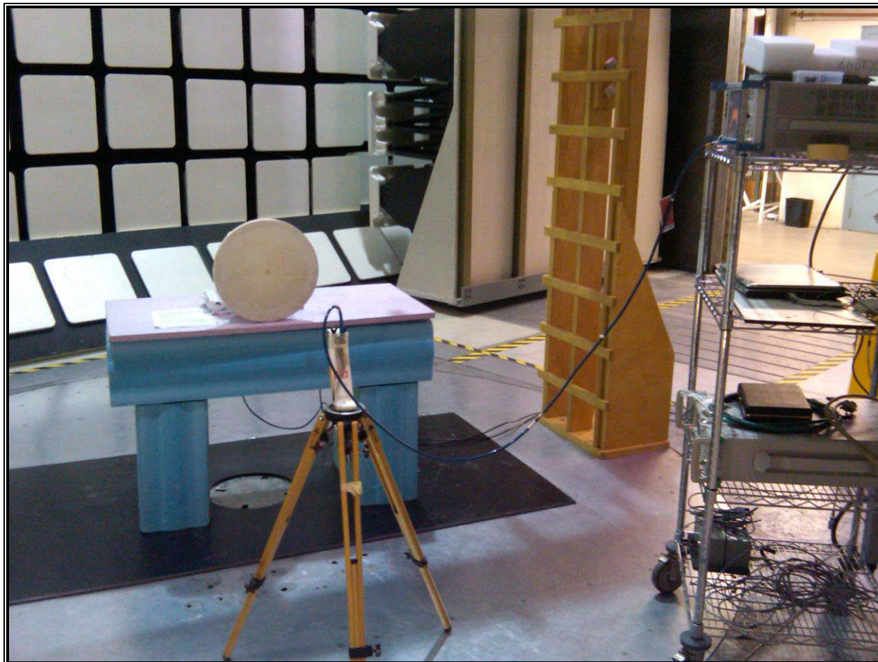
Figure 3: Setup for testing Configuration 1, 30 cm EUT antenna
