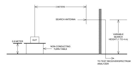
The spectrum was search up to the 10<sup>th</sup> harmonic of the fundamental frequency of operation.
