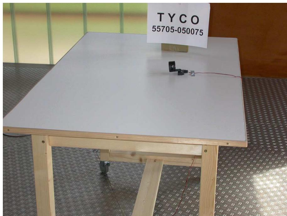
**Test setup for radiated emission measurement
