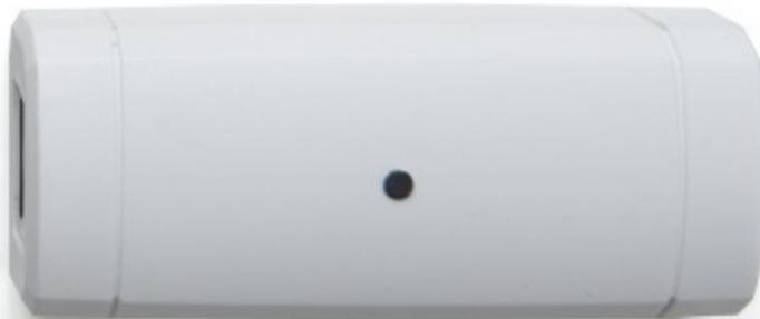
The RA-R426-01 module's transmitter functionality serves to periodically transmit short messages containing tens of bytes of information: a unique identifier and typically additional payload data. The receiver functionality serves to continuously listen for similar messages originating from compatible devices in range. For most applications, the module's transceiver is disabled more than 99% of the time.
