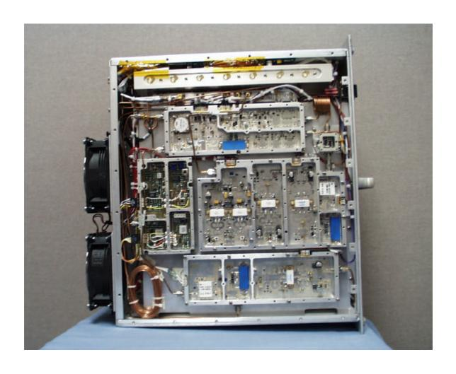
Figure: 5 MCPA SIDE VIEW – COVERS REMOVED
