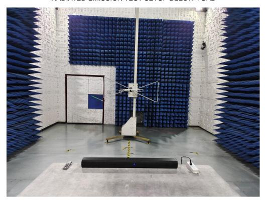
RADIATED EMISSION TEST SETUP ABOVE 1GHz
