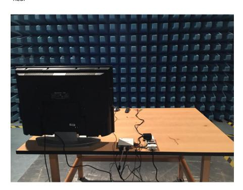
FCC Part15C Radiated Emission above 1GHz
