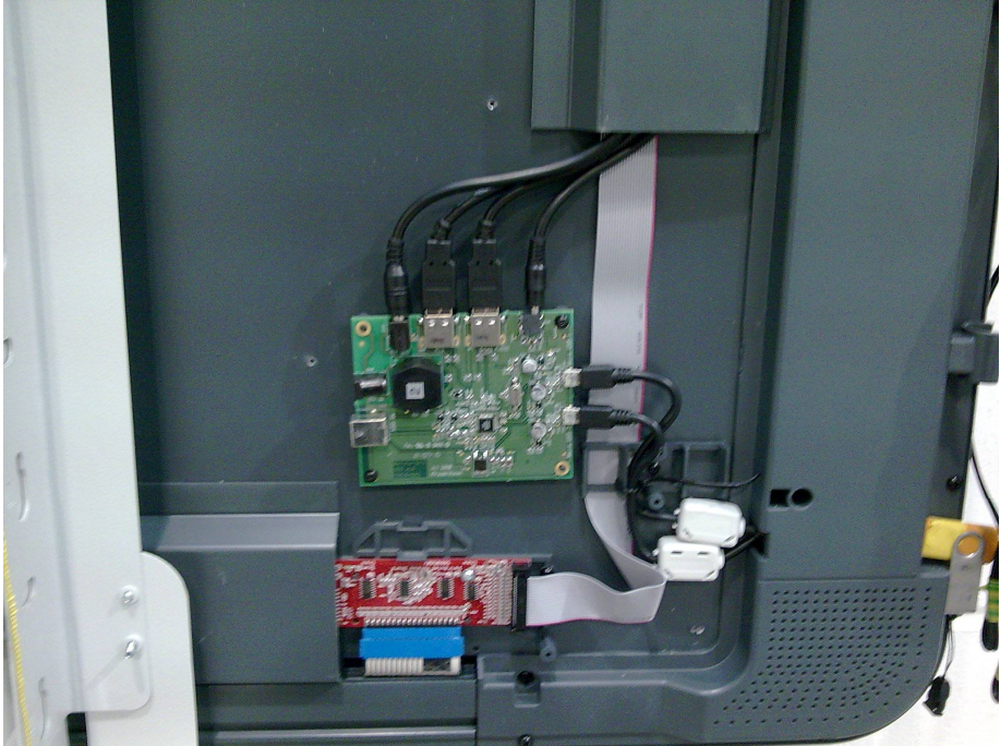
USB Hub PCB and Audio amplifier
