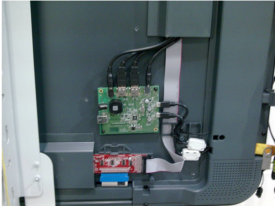
USB Hub PCB and Audio amplifier
