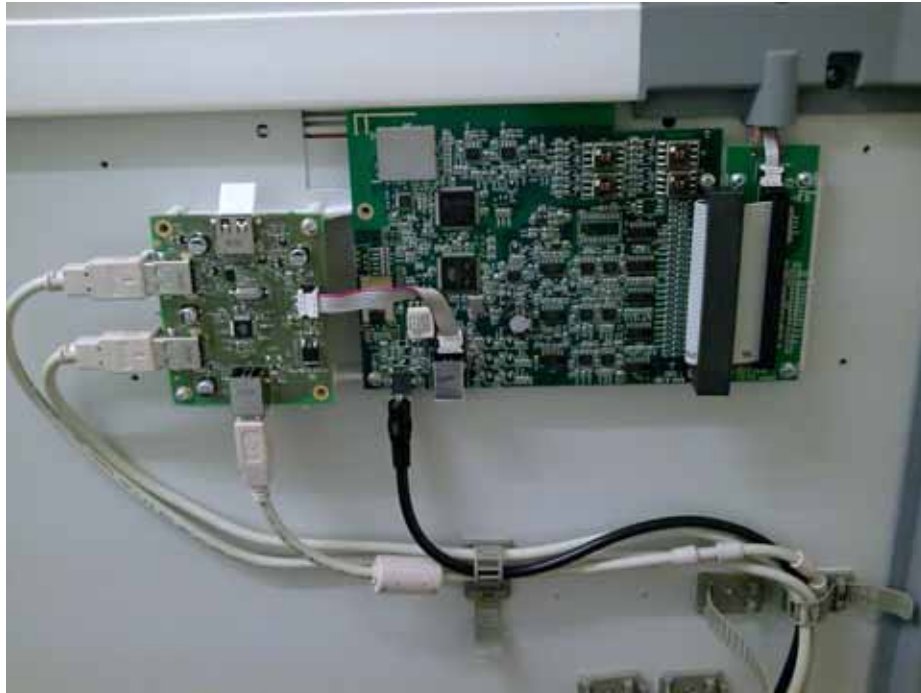
PHOTOGRAPH No. 1 2.4GHz RADIO PCB FITTED ON REAR OF BOARD HUB UNIT WITH USB AUDIO AMPLIFIER FITTED IN THE SIDE PANEL
