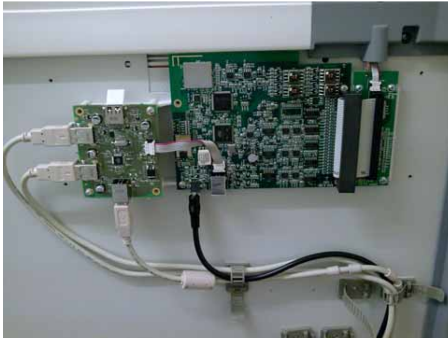
PHOTOGRAPH No. 4 2.4GHz RADIO PCB FITTED ON REAR OF BOARD HUB UNIT WITH USB AUDIO AMPLIFIER FITTED IN THE SIDE PANEL
