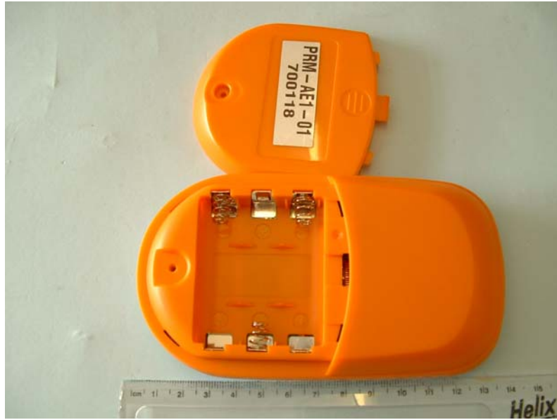
Rear Overview Battery Cover REmoved
