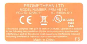
The label size is 50mm x 20mm (2mm Corner Rad), Background colour Pantone Orange 151C with text and symbols White, Lexan Polycarbonate Film 8B35 and is fully compliant with UL/IEC 60950-1 for Adhesion and Durability. The label is affixed to the rear of the Activexpression.
