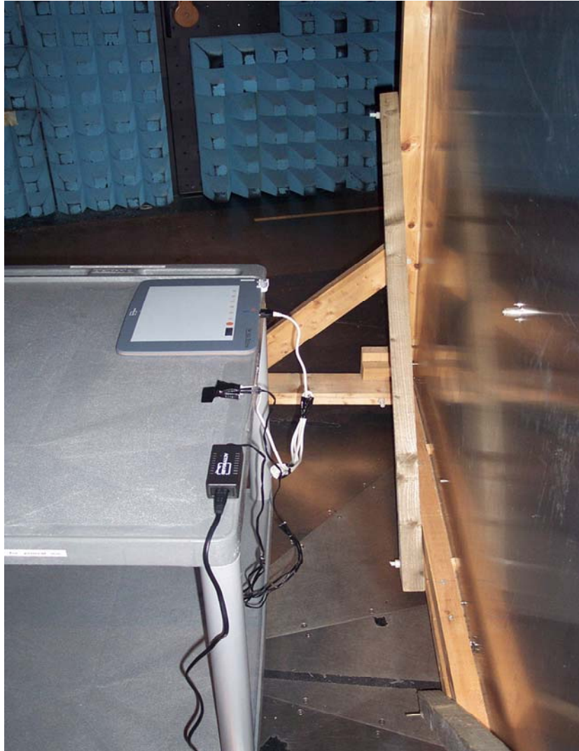
Conducted Emissions on Power Lines Set Up Photograph
