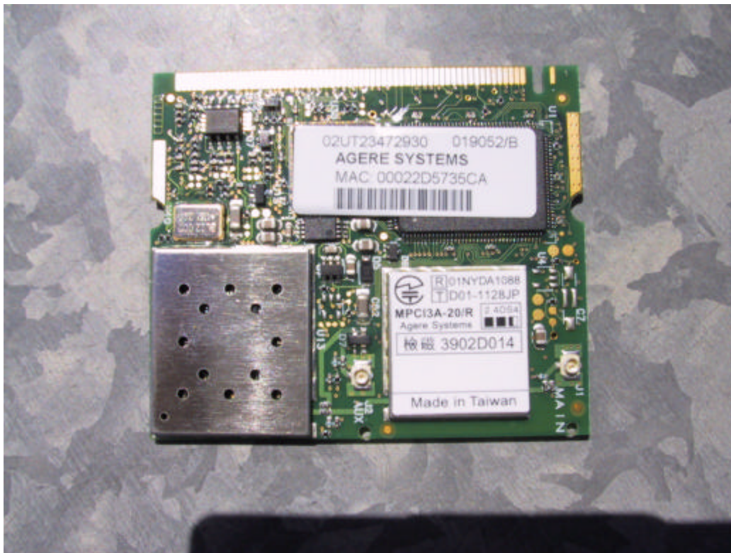
Radio PCB Top Side
