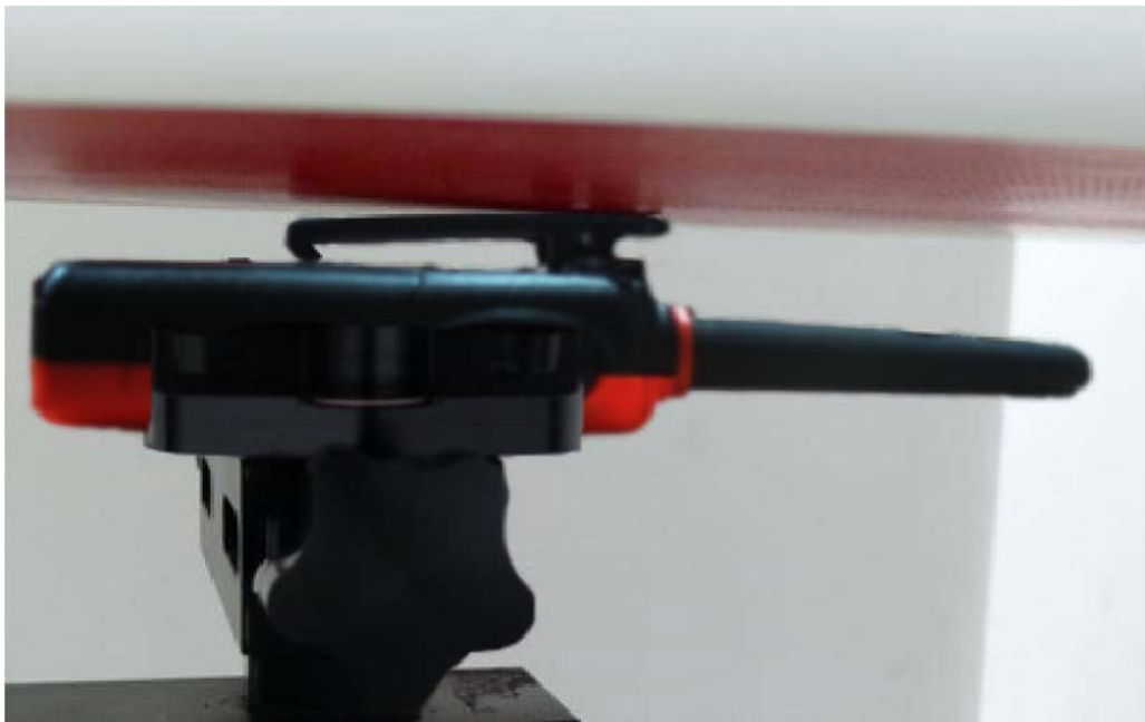
Picture 5: Body, The EUT display towards ground, Belt clip attach the Panntom
