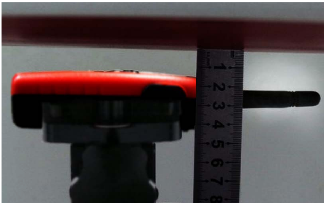
Picture 4: Body, The EUT display towards phantom, the distance from EUT to the bottom of the Phantom is 15mm
