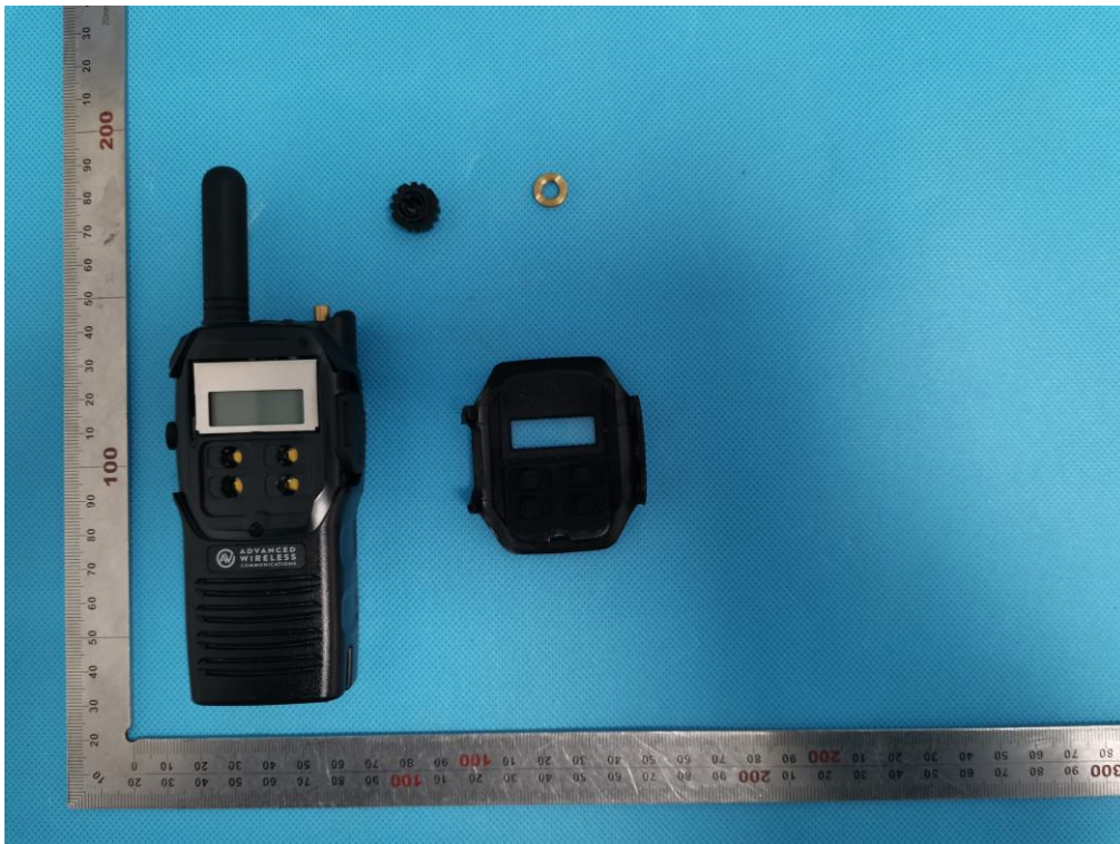
OPEN VIEW OF EUT (FIGURE 2)
