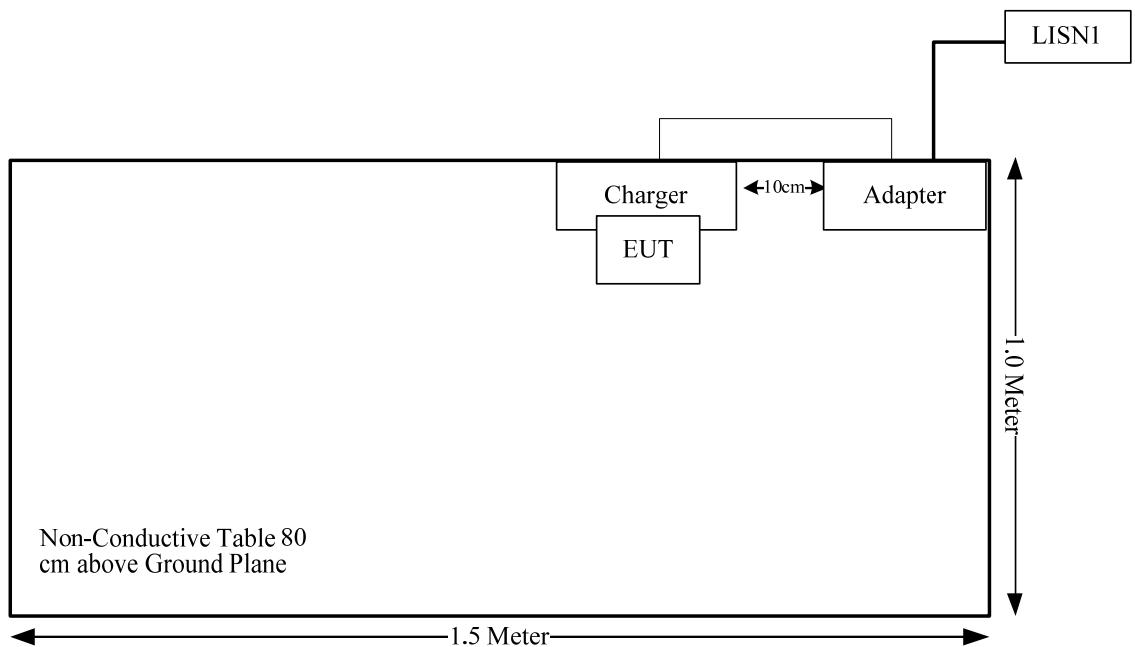
Radiation Emissions Test For Below 1GHz:
