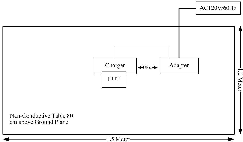
Radiation Emissions Test For Above 1GHz:
