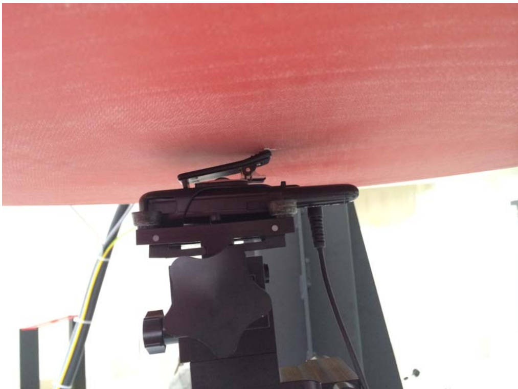
Body-worn, the front of the EUT towards ground with A1, B2, BC2 and AA1 (The distance was 0cm)
