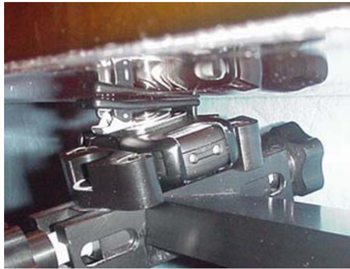
Belt-Clip Swivel Position #2 = -90 Degrees Antenna Distance to Planar Phantom = 1.0 cm
