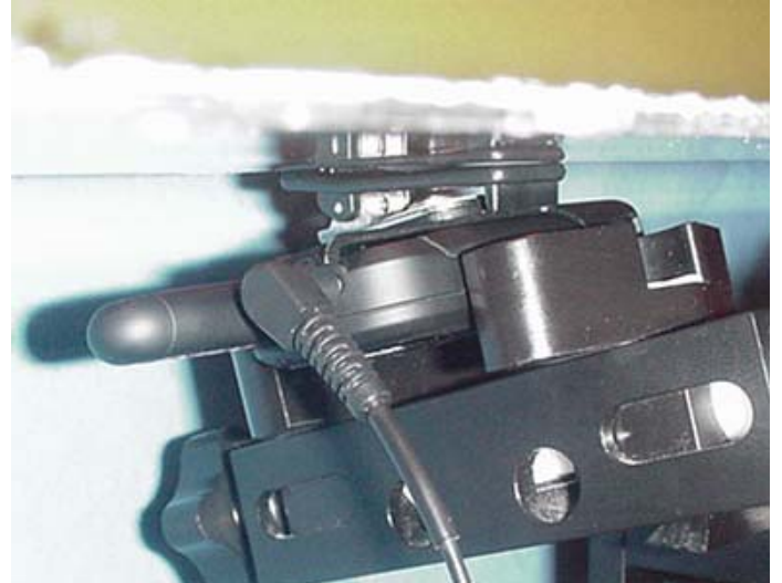
Belt-Clip Swivel Position #3 = 90 Degrees Antenna Distance to Planar Phantom = 2.0 cm
