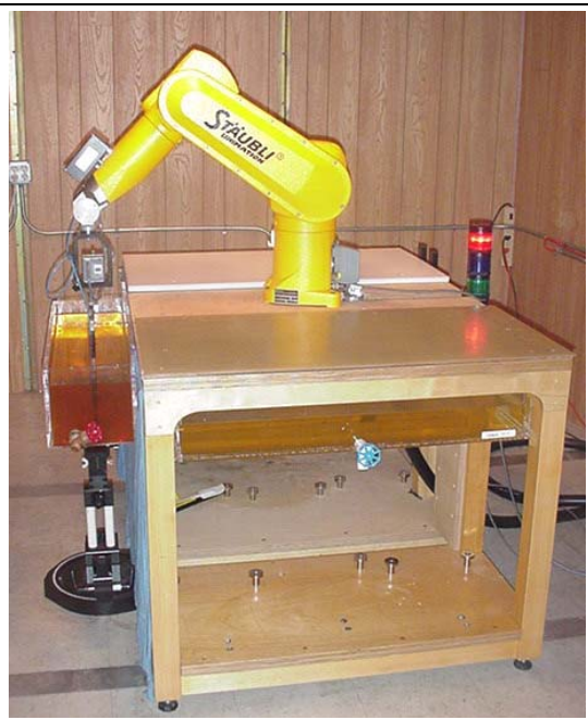
DASY4 System with Plexiglas side planar phantom
