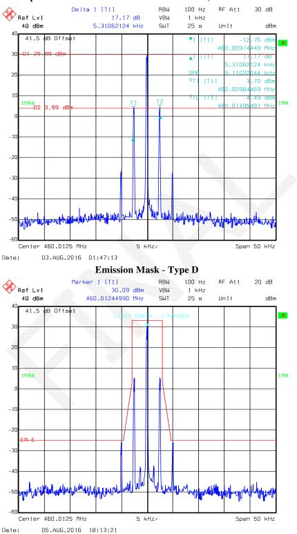
Occupied Bandwidth -6.25 kHz 460.0125 MHz, Low Power Level
