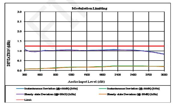
Note: For channel spacing: 6.25 kHz, the full system rated deviation is 1.25 kHz which specified by manufacturer.
