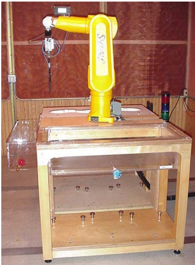
DASY4 SAR Measurement System with validation phantom
