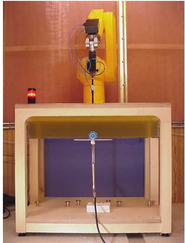
DASY3 SAR Measurement System with validation phantom
