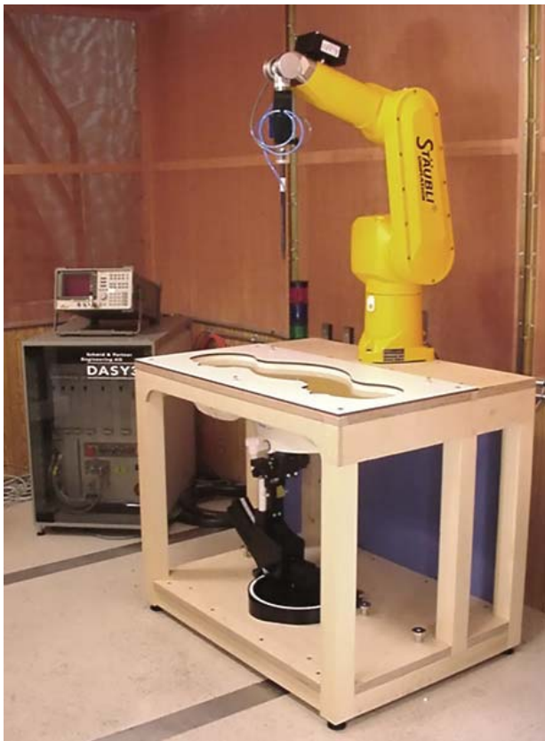
DASY3 SAR Measurement System with SAM Phantom
