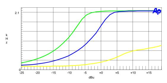
**Modulation Limiting Plots:** Green (2.5KHz), Blue (1.0KHz), and Yellow (300Hz)
