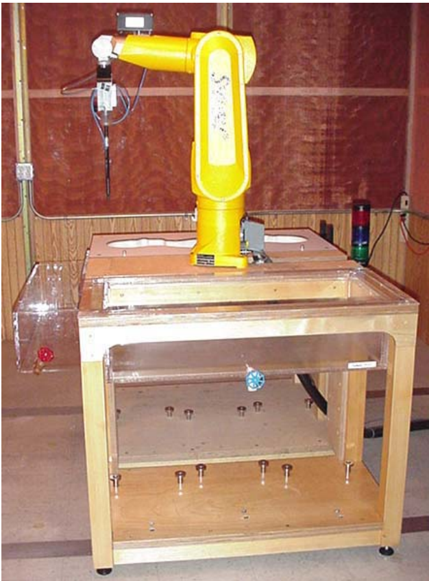
DASY4 SAR Measurement System with validation phantom
